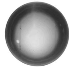
DT ice layer in the foam capsule -1-μm-rms roughness
